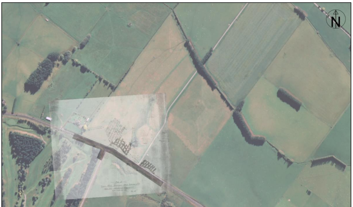
Figure 2: Georeferencing of old mine workings on the southern perimeter of the study area. The mine workings are primarily underground.
