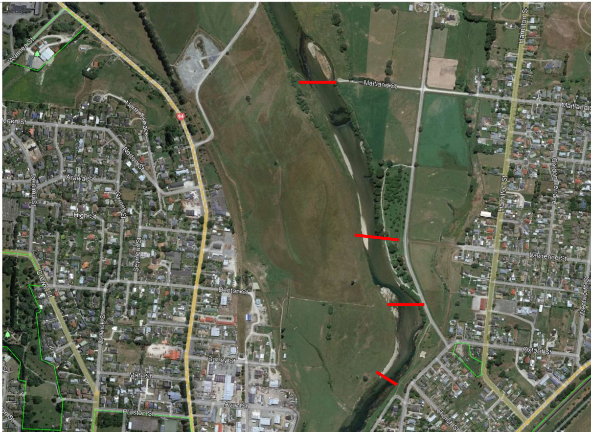
Figure 2-2 Northern Region Bridge Options. From South to North: 1) Surrey Street (2021 option) 2) Denton Street 3) Lawrence Street 4) Maitland Street. Bridge options requiring at least one approach ramp constructed on the flood plain.
