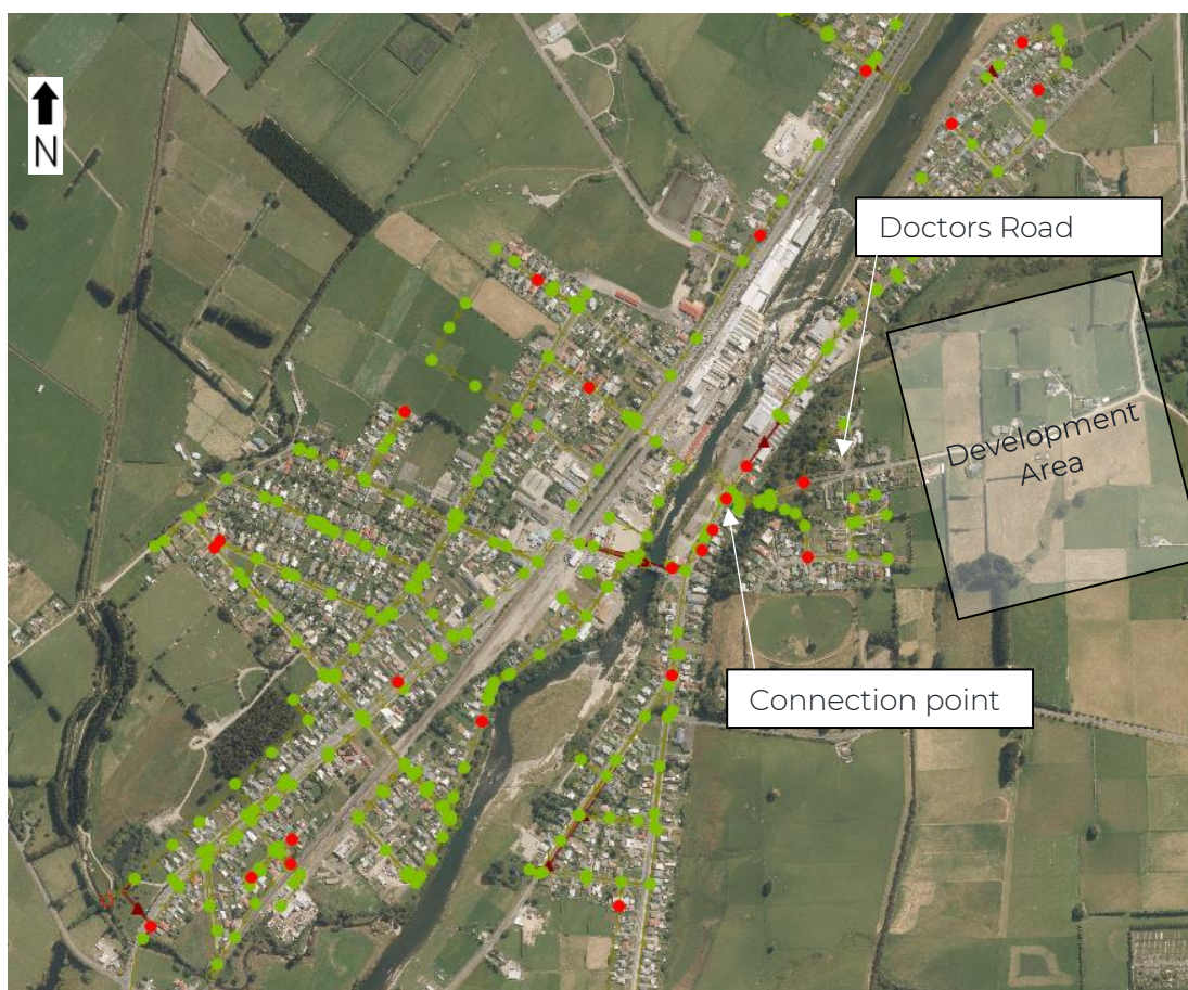
Figure 5-4: Location of 28 manholes where there was a predicted increase in spill volume greater than 1% during a 50% AEP 1-hour design rainfall event.
