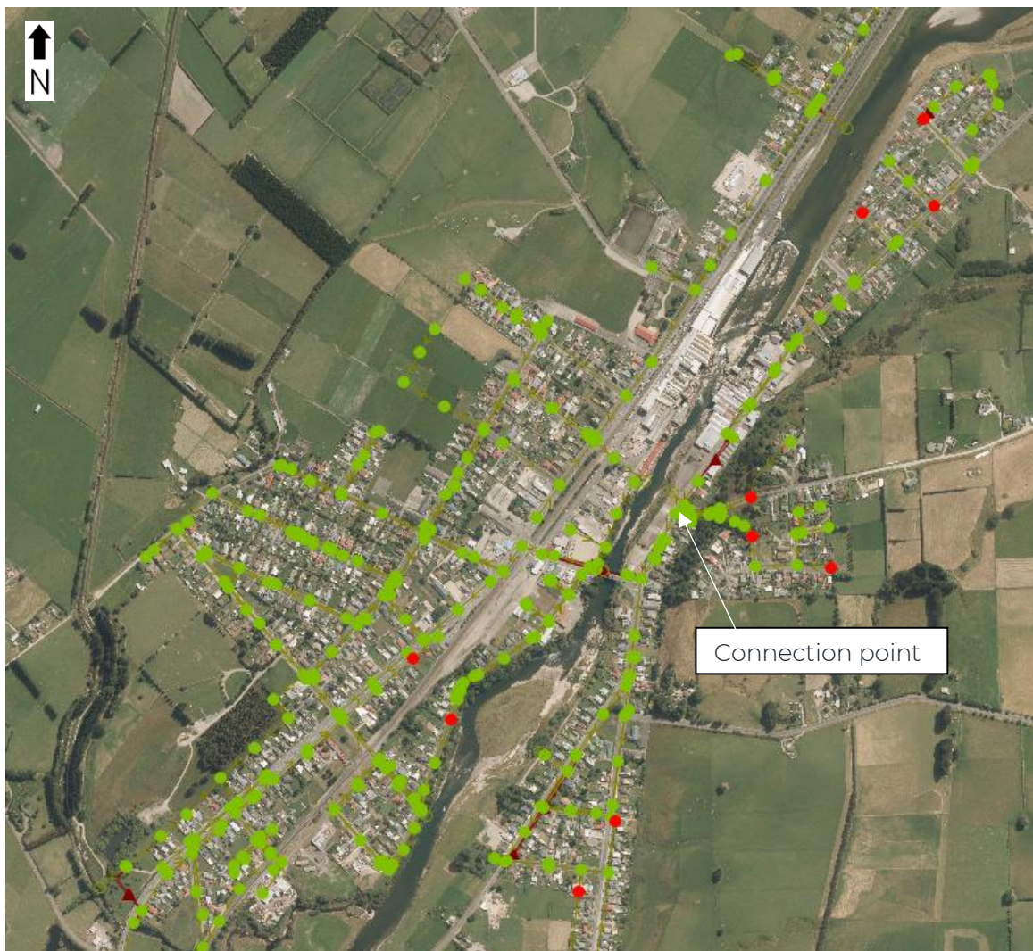
Figure 7-9. Manhole with spill volumes that increase from baseline following upgrades.
