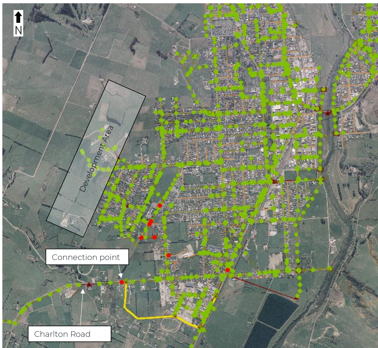
Figure 5-3. Location of manholes where there is a predicted increase in spill volume during a 50% AEP 1-hour design rainfall event in Gore.
