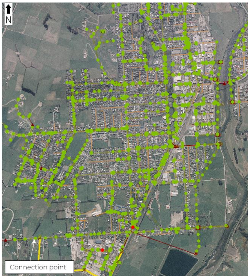
Figure 7-3. Manhole with spill volumes that increase from baseline following upgrades.
