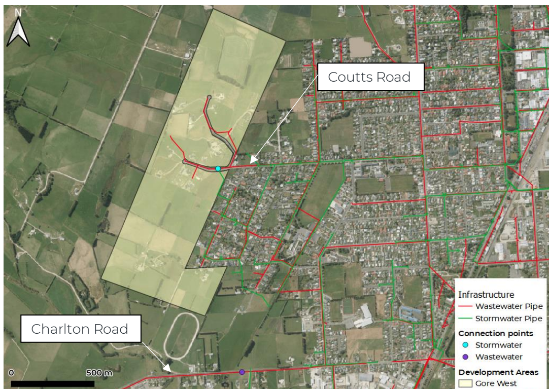
Figure 4-6. Gore residential development connection point.
