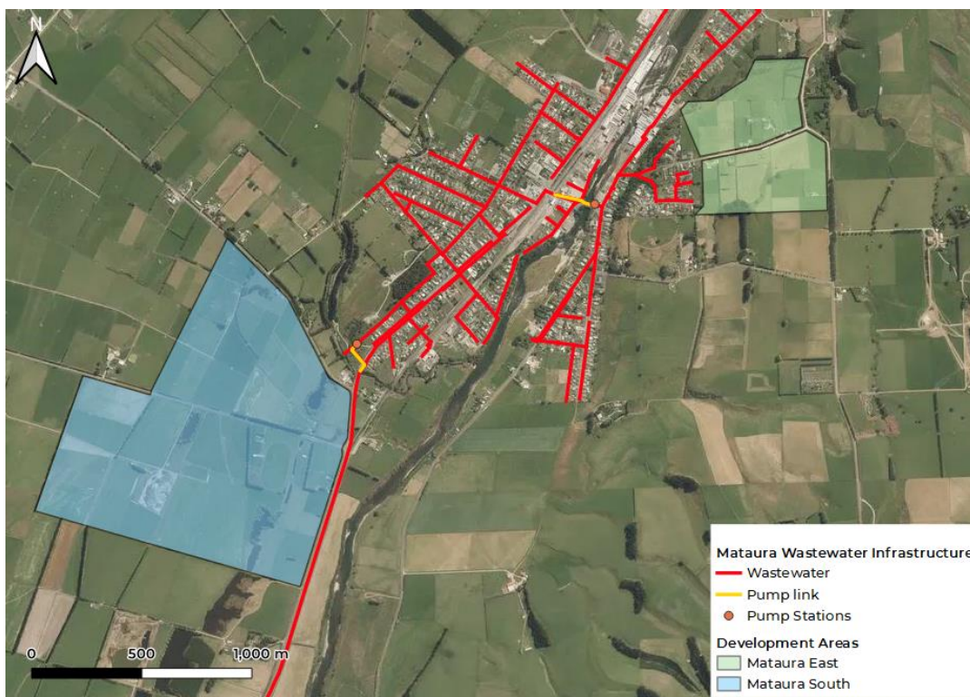
Figure 4-1. Matura Wastewater System Overview
