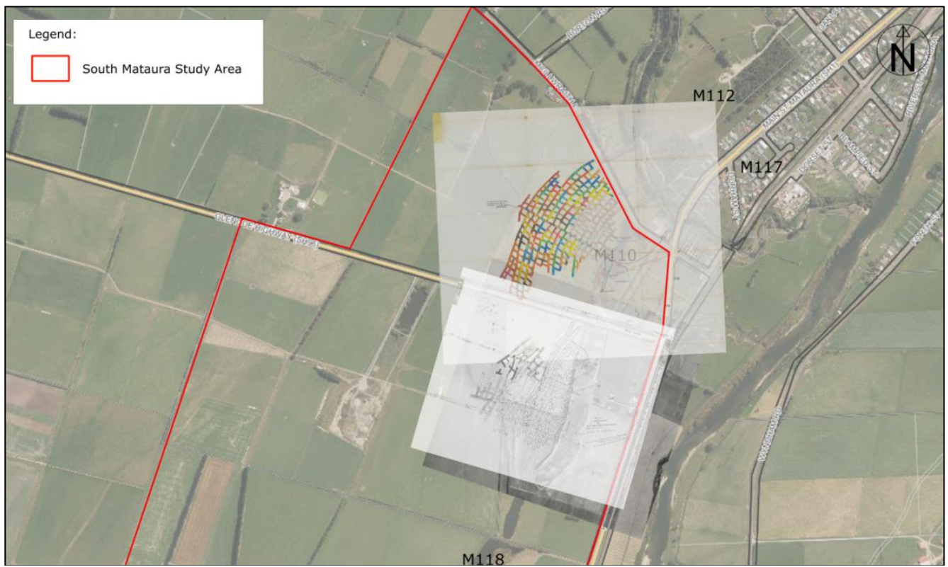
Figure 2: Georeferencing of the underground mine workings for the northern extent of the Study area, no other underground mining was found during this review.
