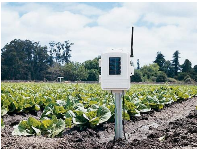
Figure 3 - Leaf and soil moisture temperature station
