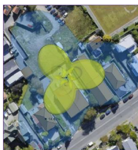
An example of RF Lobes – Plan view
